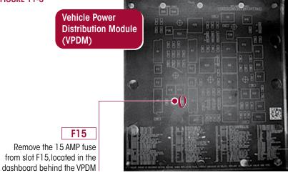
Prior to service of the lift axle, adjacent components or the air controller module:
