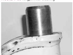
2. Inspect the kingpin for wear or damage. Use a micrometer and measure the upper and lower kingpin in two locations. Positions must be 90° opposed from each other. If the kingpin has less than 1.802" diameter, replacement of the axle is necessary, see Figures 9-34 through 9-37.
