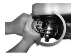
10. Position yourself directly below the tie rod end. Using both hands, grab the assembly end as close to the tie rod end as possible (no more than 6" or 152.4 mm). Apply hand pressure with reasonable human effort vertically up and down in a push-pull motion several times (using approx. 50-100 lbs. of force). Check for any movement or looseness at both tie rod end locations, see Figure 7-9.
