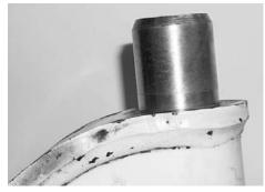
Inspect the kingpin for wear or damage. Use a micrometer and measure the upper and lower kingpin in two locations. Positions must be 90° opposed from each other. If the kingpin has less than 1.802" diameter, replacement of the axle is necessary, see Figures 9-37 through 9-40.
