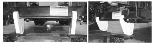
Prior to lifting the vehicle, ensure that the bottom axle plate is flat in the tow fork to minimize any gap between the bottom axle plate and the tow fork. See Figure 6-5 and 6-6.
