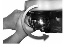
9. Position yourself directly below the tie rod end. Using both hands, grab the assembly end as close to the tie rod end as possible (no more than six inches or 152.4mm). Apply hand pressure with reasonable human effort vertically up and down in a push-pull motion several times (using approximately 50-100 pounds of pressure). Check for any movement or looseness at both tie rod end locations. See Figure 7-5.
