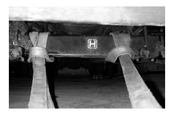
FIGURE 6-8 CHAINS ARE NOT ACCEPTABLE FOR OFF ROADWAY TOWING
