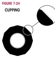
**Cupping** — Localized, dished out areas of fast wear creating a scalloped appearance around the tire. Cupping, which appears around the tire on the shoulder ribs, may also progress to adjoining ribs, see TMC RP 219A publication, page 7.
