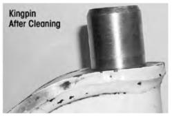
2. Inspect the kingpin for wear or damage. Use a micrometer and measure the upper and lower kingpin in two locations. Positions must be 90° opposed from each other. If the kingpin has less than 1.802" diameter, replacement of the axle is necessary, see Figures 9-26 through 9-29.
