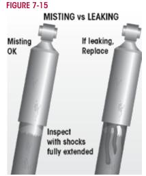
when the shock absorber is fully extended, underneath the main body (dust cover) of the shock absorber. Look for these potential problems when doing a visual inspection. Inspect the shock absorbers fully extended. Replace as necessary.
