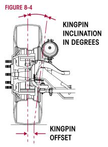
**Kingpin Inclination (KPI)** — The inward tilt of the kingpin from the vertical. This front suspension parameter has a pronounced effect on steering effort and return ability. As the front wheels are turned around an inclined kingpin, the front of the truck is lifted. This lifting of the vehicle is experienced as steering effort when the turn is executed and exhibits itself as recovery force when the steering wheel is released.
