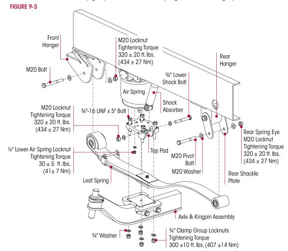
15. Lower the jack allowing the suspension to pivot down out of the rear hanger clamps.
