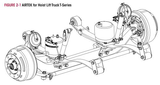
**AIRTEK** — AIRTEK is an integrated front air suspension and fabricated steer axle that work together to form an integrated torsion system. This lightweight system provides driver comfort and is ideal for a variety of applications. Utilizing a system approach, Hendrickson has engineered and optimized the following components to form a system delivering superior ride, stability and handling characteristics with reduced weight and maintenance.
