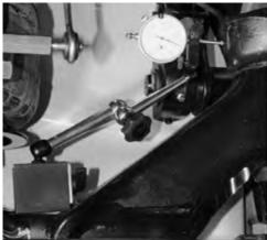
FIGURE 7-18 CHECKING LOWER KINGPIN BUSHING
