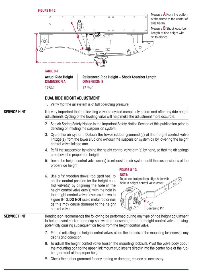
10. Facing the air spring from the outboard side for the left side of the vehicle, pivot the valve body counter clockwise to increase the ride height and clockwise to decrease the ride height. For the right side of the vehicle, pivot the valve body clockwise to increase the ride height and counter clockwise to decrease the ride height.
