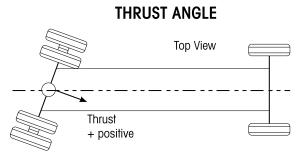
**Thrust Angle, Tracking, or Square** — The angle formed by the centerline of the vehicle frame (geometric centerline) and the direction that an axle points. As indicated by the term "square", the ideal value for the angle is 0° or when the axle centerline is at 90° or perpendicular to the geometric centerline. Thrust or tracking to the right is positive, and to the left is negative.
