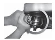
10. Position yourself directly below the tie rod end. Using both hands, grab the assembly end as close to the tie rod end as possible (no more than 6" or 152.4mm). Apply hand pressure with reasonable human effort vertically up and down in a push-pull motion several times (using approximately 50-100 pounds of force). Check for any movement or looseness at both tie rod end locations, see Figure 7-6.
