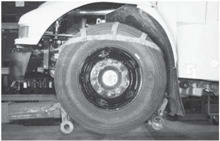
FIGURE 6-1 Wheel lift method
