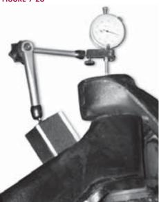
of the upper steering knuckle to obtain the proper clearance specification. See Steering Knuckle Assembly in the Component Replacement Section of this publication for proper shim installation.
