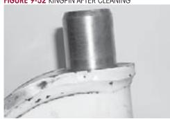
2. Inspect the kingpin for wear or damage. Use a micrometer and measure the upper and lower kingpin in two locations. Positions must be 90° opposed from each other. If the kingpin has less than 1.802" diameter, replacement of the axle is necessary, see Figures 9-53 through 9-56.
