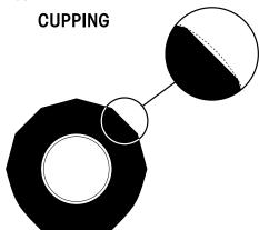
**Cupping** — Localized, dished out areas of fast wear creating a scalloped appearance around the tire. Cupping, which appears around the tire on the shoulder ribs, may also progress to adjoining ribs, see TMC RP 219A publication, page 7.
