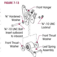
If one thrust washer is worn out, Hendrickson recommends both thrust washers on that side of the suspension be replaced. Inspect the thrust washers on the other side of the vehicle and replace if necessary.
