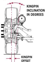
**Kingpin Inclination** — The inward tilt of the kingpin from the vertical. This front suspension parameter has a pronounced effect on steering effort and returnability. As the front wheels are turned around an inclined kingpin, the front of the truck is lifted. This lifting of the vehicle is experienced as steering effort when the turn is executed and exhibits itself as recovery force when the steering wheel is released.
