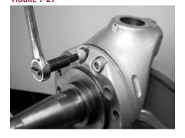
2. Retighten the socket head cap screws to **1**75-200 foot pounds torque.
