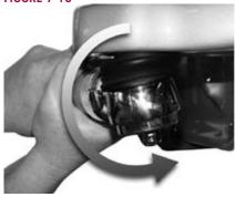
10. Position yourself directly below the tie rod end. Using both hands, grab the assembly end as close to the tie rod end as possible (no more than 6" or 152.4 mm). Apply hand pressure with reasonable human effort vertically up and down in a push-pull motion several times (using approximately 50-100 foot pounds of force). Check for any movement or looseness at both tie rod end locations, see Figure 7-11.
