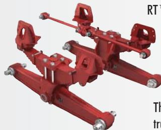
RT™ / RTE™ Series is a durable steel spring suspension with a legacy of over 70 years of reliability in the most severe applications. Hendrickson-designed springs provide a consistent spring rate for longer life as the equalizing beams distribute load equally between both axles for improved traction. The system performs well in a variety of vocational truck applications.
