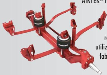
AIRTEK® represents a quantum leap in front suspension and axle technology. This product offers unmatched ride and handling performance with up to 55 lbs. of weight savings and reduced maintenance requirements. AIRTEK utilizes STEERTEK, Hendrickson's patented fabricated steer axle.
