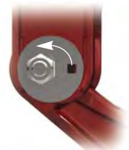
QUIK-ALIGN® — Rotating the eccentric collar allows up to 1 inch of axle alignment per side
