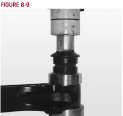
4. Place the torque rod bushing centered in the assembly funnel, see Figure 8-9. The bar pin must have the mounting flats positioned as indicated in Figure 8-10.
