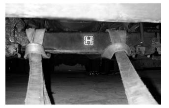
FIGURE 6-8 CHAINS ARE NOT ACCEPTABLE FOR OFF ROADWAY TOWING
