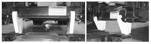
Prior to lifting the vehicle, ensure that the bottom axle plate is flat in the tow fork to minimize any gap between the bottom axle plate and the tow fork, see Figure 6-5 and 6-6.
