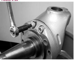
7. Remove the upper steering knuckle by sliding it up off the kingpin.
