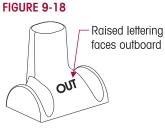
7. Install the shock absorbers on 5/8" lower shock mounting bolts. Install the washers and locknuts and tighten per vehicle manufacturer's torque specifications.
