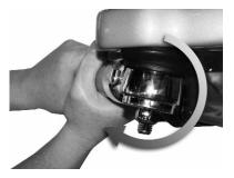
10. Position yourself directly below the tie rod end. Using both hands, grab the assembly end as close to the tie rod end as possible (no more than 6" or 152.4mm). Apply hand pressure with reasonable human effort vertically up and down in a push-pull motion several times (using approx. 50-100 pounds of force). Check for any movement or looseness at both tie rod end locations, see Figure 7-7.
