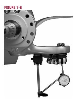
According to the Commercial Vehicle Safety Alliance (CVSA), the "out of service" criteria for any commercial vehicle is: Any motion other than rotational between any linkage member and its attachment point of more than <sup>1</sup>/8" (3mm) measured with hand pressure only. (393.209(d)), (published in the North American Standard Out-of-Service Criteria Handbook, April 1, 2006.)
