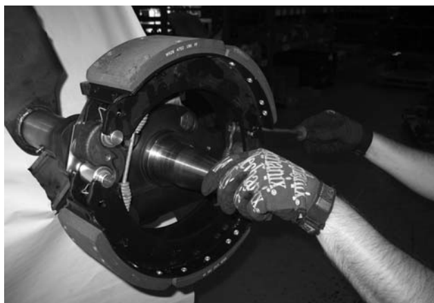
Figure 46. Removal of Outer and Inner Retaining Spring
