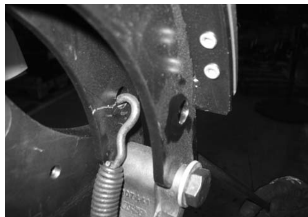
Figure 49. Spring Clipped Completely Into Mounting Hole
