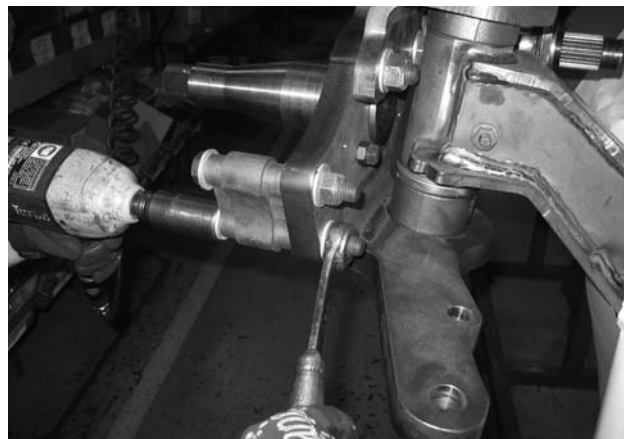
Figure 48. Removal of Brake Bolts and Anchor Pin
