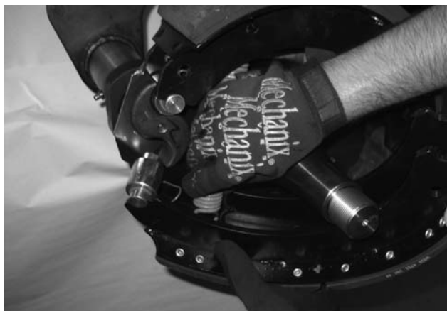
Figure 47. Removal of Return Spring
