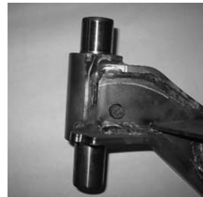
Figure 22. Kingpin After Cleaning
