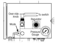
Lift Mode D (Down when vehicle ignition is off) **Remote Operation** (via electric switch)
