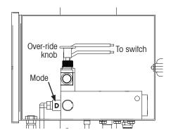
**NOTE:** AKADO008/AKAD2010-2 (air line in port 7) control disables lift axle service brakes when in raised
