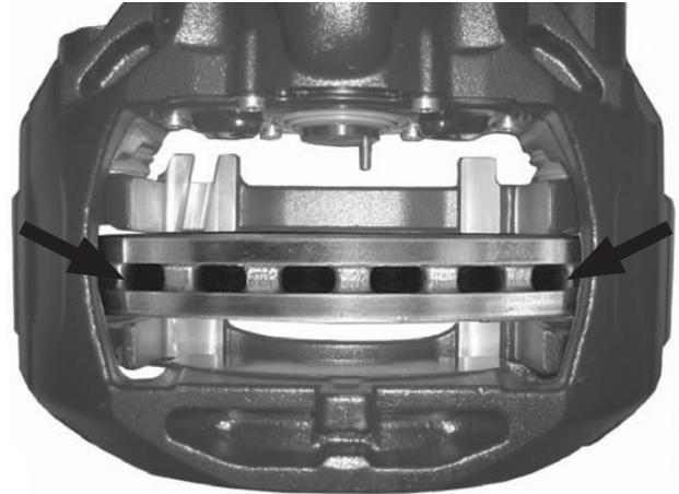
Figura 40: Positioning caliper over brake rotor
