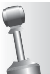
Damaged dust cover and / or shock body
