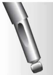
Bent or dented shock
