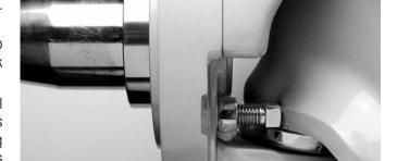
turned to the full lock position for each right hand and left hand direction. Refer to the vehicle manufacturer for exact specifications.
