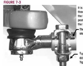
It is critical that the threaded portion of the tie rod end extends past the slots into the tie rod tube.
