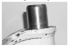
Inspect the kingpin for wear or damage. Use a micrometer and measure the upper and lower kingpin in two locations. Positions must be 90° opposed from each other. If the kingpin has less than 1.802" diameter, replacement of the axle is necessary, see Figures 9-7 through 9-10.
