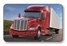
SOFTEK® NXT system combines the STEERTEK™ NXT axle and monoleaf spring technology with an advanced integrated clamp group design and is now available with Integrated Air Disc Brake (IADB) knuckles for greater weight savings.
