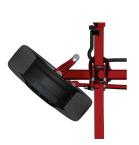
Optimized steering system – 55-degree wheel cut
